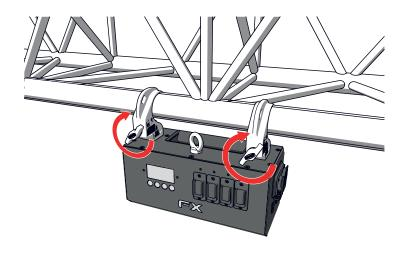
3 Secure the MAGICFX® SWITCHPACK onto the truss with use of the safety eye.
