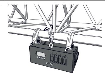
4 Inspect if the MAGICFX® FX-SWITCHPACK is mounted firmly and secured correctly.
